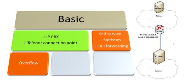
The Basic product profile is the simplest set-up option in the SIP Trunk product. The SIP Trunk is set up using one connection point to Telenor, one fixed IP-PBX Host IP address and a fixed port.
