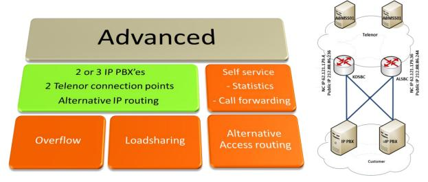
With the Advanced product profile, the SIP Trunk is set up using two connection points to Telenor, two or three fixed IP-PBX Host IP addresses and a fixed port.
